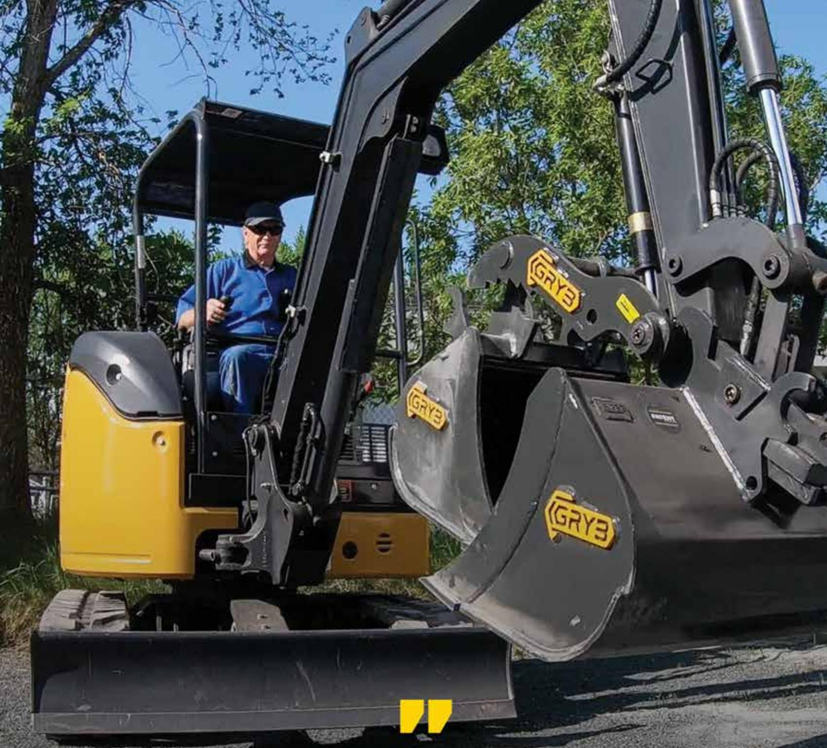
**The main advantage of the hydraulic quick attach is the ease with which you can change your bucket. You can do it with a simple push of a button.**
